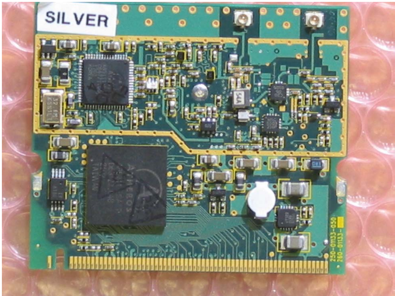
RF Module, Side 1, w/o shield
