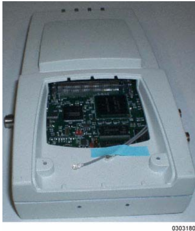
Figure - Airespace AP with Door Removed
