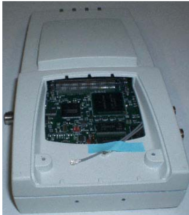
Figure - Airespace AP with Door Removed
