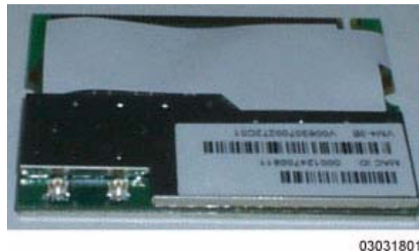
Figure - Typical Airespace AP 802.11a Radio Card
