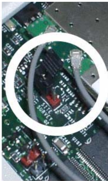
A. Site Survey Jumper Not Installed
