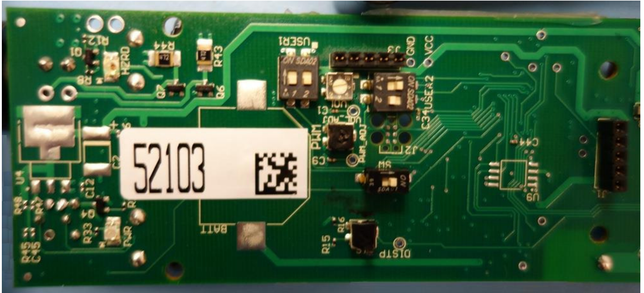
Magnetic Field Generator-Internal Photo Generator/Receiver Board-Bottom View (pt. 2)
