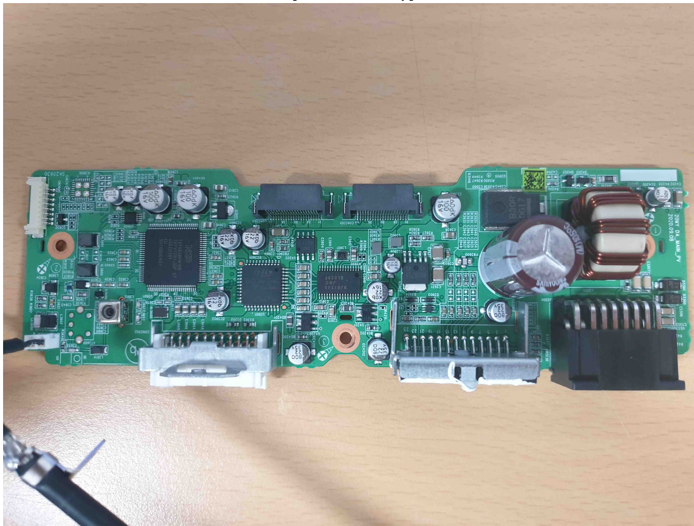
[Power Board Top]
