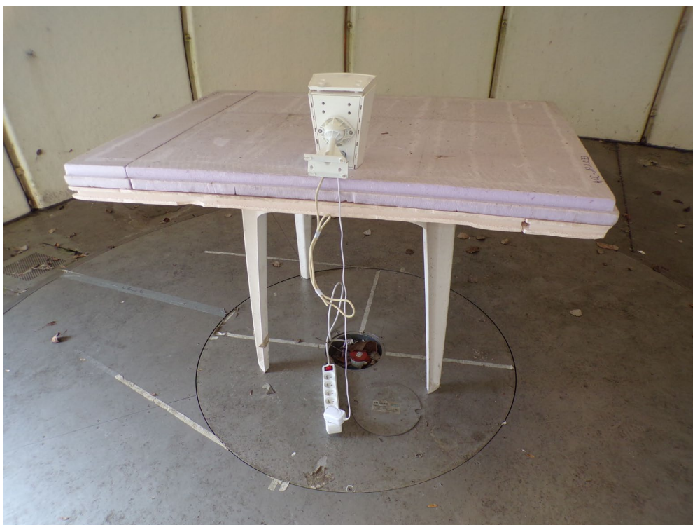
Open Area Test site (30M-1GHz)
