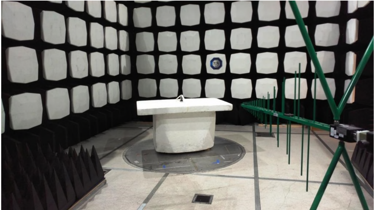
Figure 4: Equipment Under Test – Radiated Emissions <1GHz
