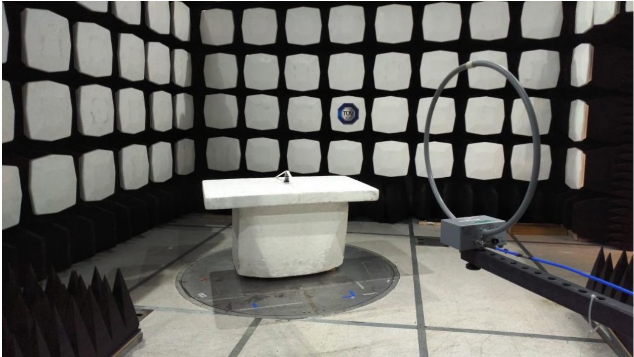
Figure 2: Equipment Under Test – Radiated Emissions <30MHz
