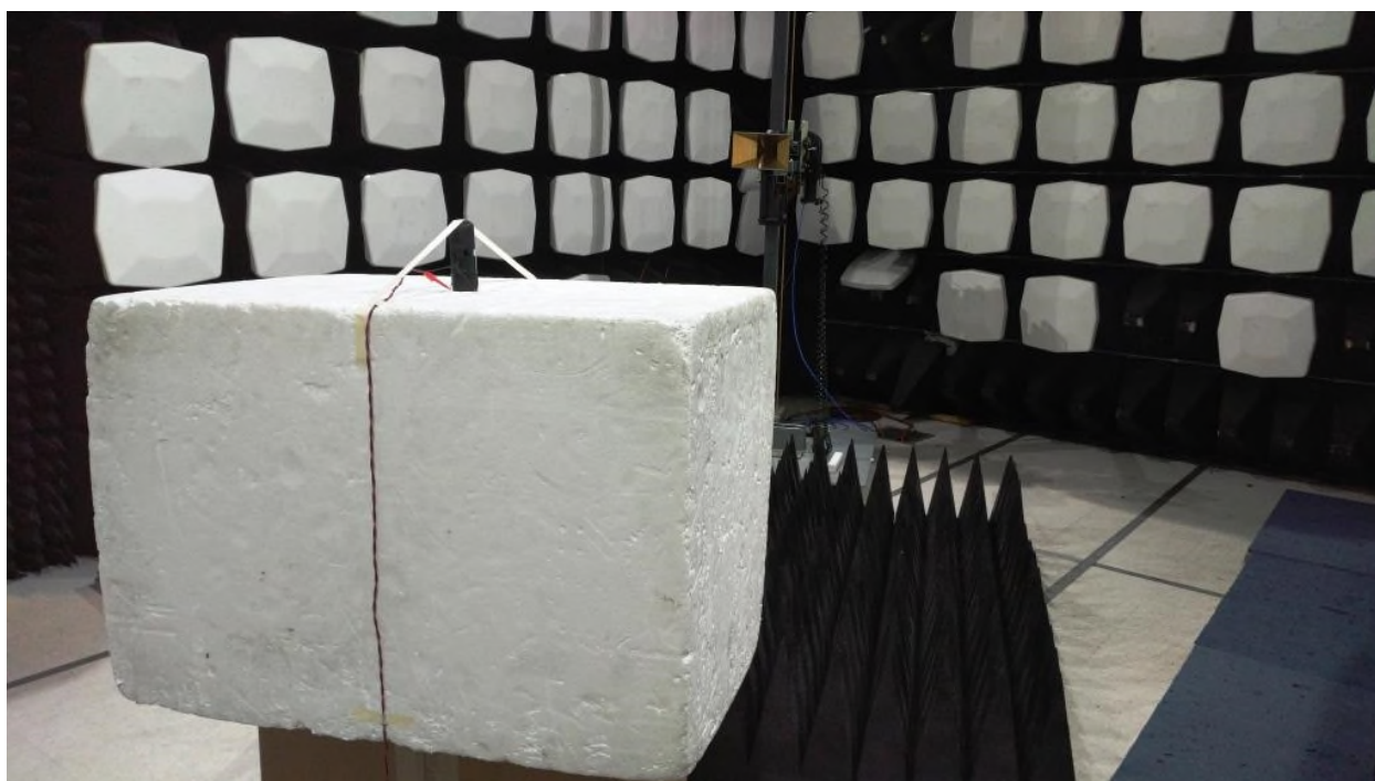
Figure 7: Equipment Under Test – Radiated Emissions >1GHz
