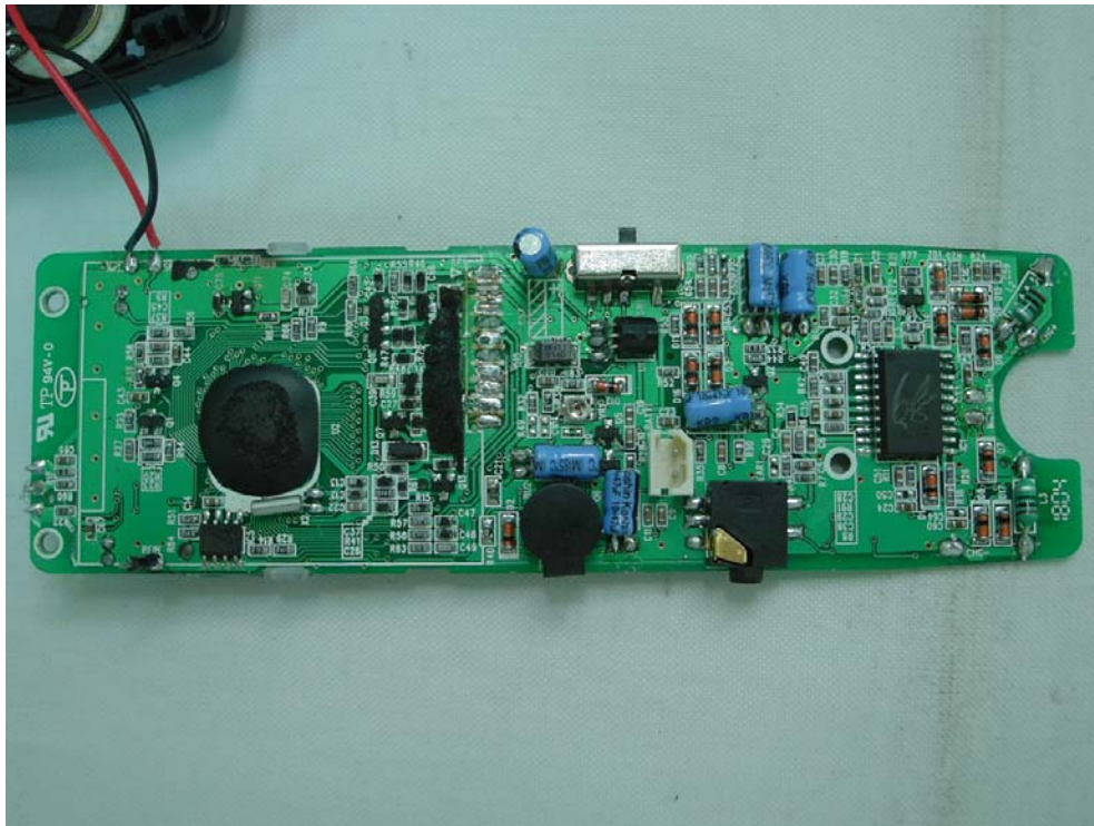
Main controller Front
