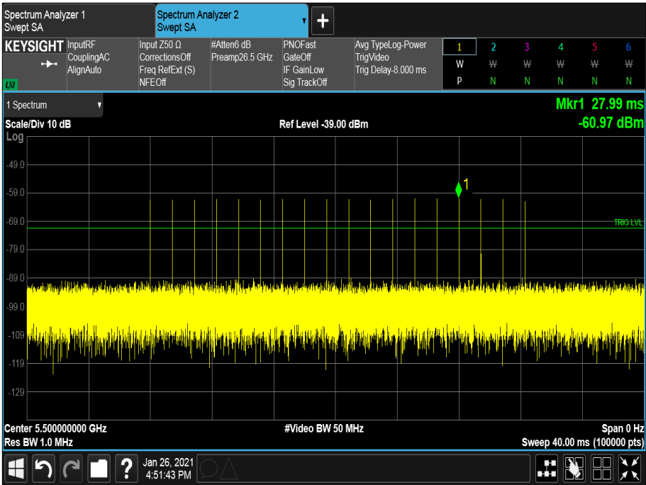
Figure 2 - Verification of Radar Type 0
