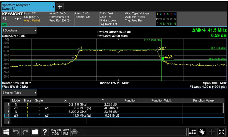
Figure 70 - Aux (B) 5230 MHz (CH46) 26 dB and 99% Bandwidth
