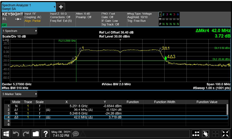
Figure 110 - Aux (B) 5270 MHz (CH54) 26 dB and 99% Bandwidth
