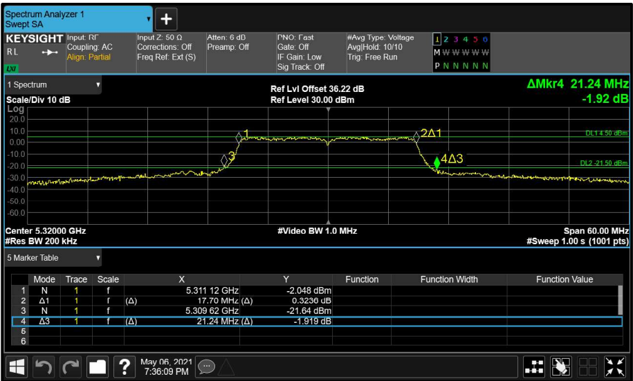
Figure 98 - Aux (B) 5320 MHz (CH64) 26 dB and 99% Bandwidth
