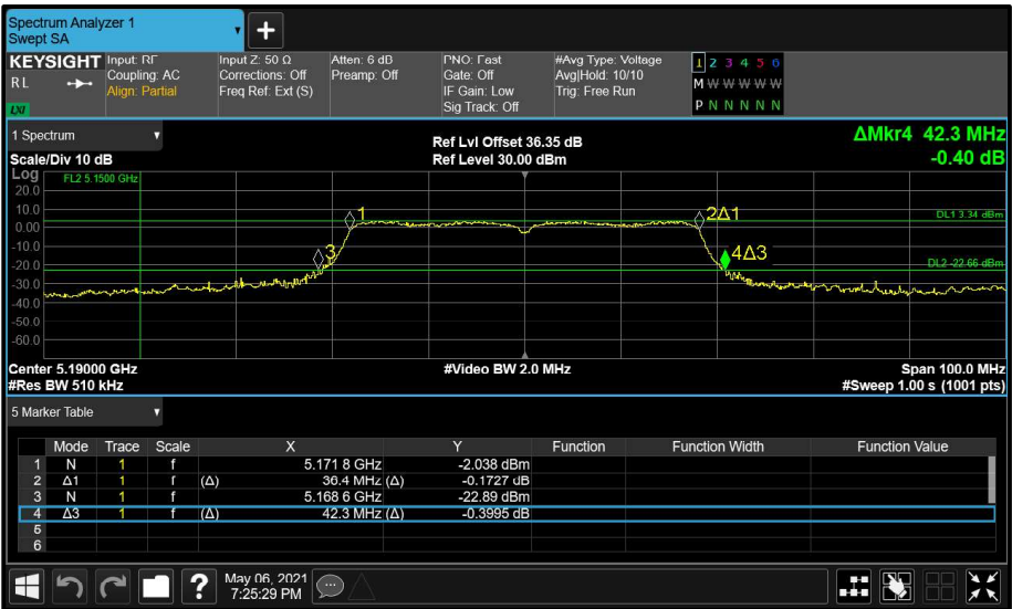
Figure 68 - Aux (B) 5190 MHz (CH38) 26 dB and 99% Bandwidth
