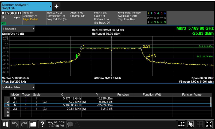
Figure 58 - Aux (B) 5180 MHz (CH36) 26 dB and 99% Bandwidth
