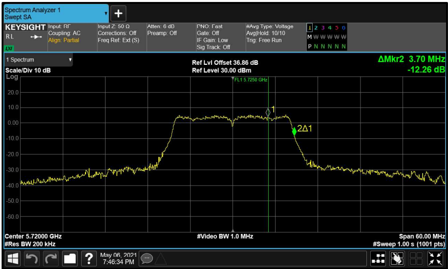
Figure 171 - Aux (B) 5720 MHz (CH144) 99% Bandwidth
