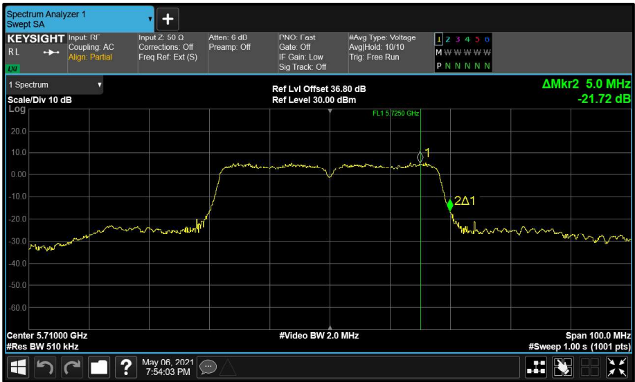
Figure 219 - Aux (B) 5710 MHz (CH142) 99% Bandwidth
