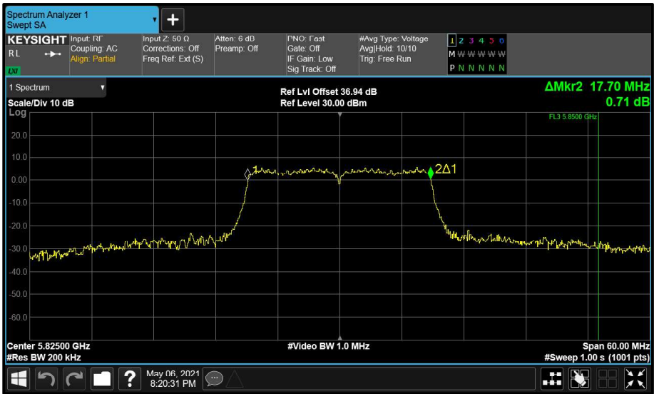
Figure 213 - Main (A) 5825 MHz (CH165) 99% Bandwidth
