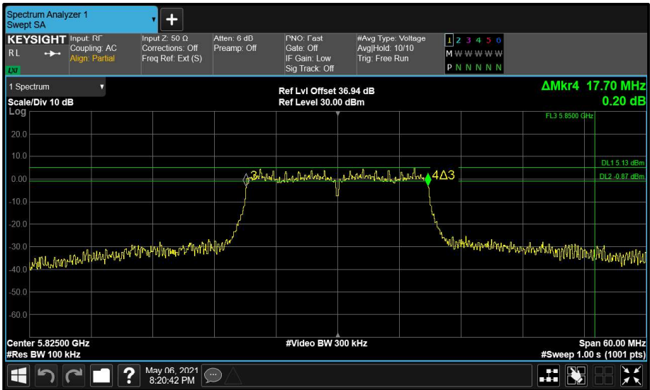
Figure 214 - Main (A) 5825 MHz (CH165) 6 dB Bandwidth
