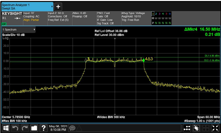
Figure 180 - Aux (B) 5785 MHz (CH157) 6 dB Bandwidth
