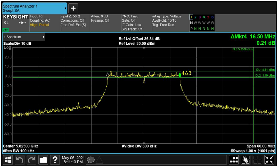
Figure 184 - Aux (B) 5825 MHz (CH165) 6 dB Bandwidth
