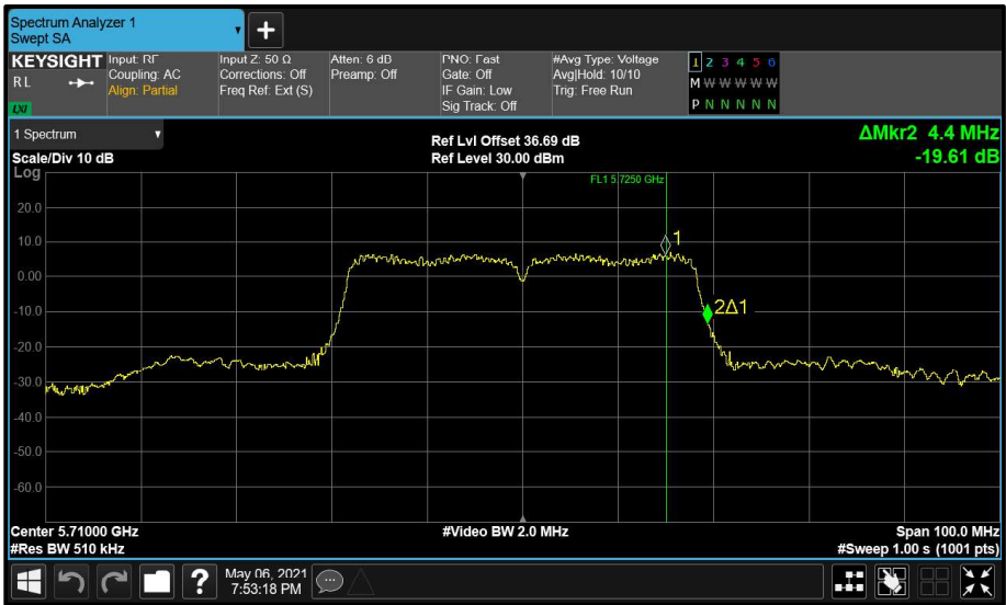
Figure 217 - Main (A) 5710 MHz (CH142) 99% Bandwidth
