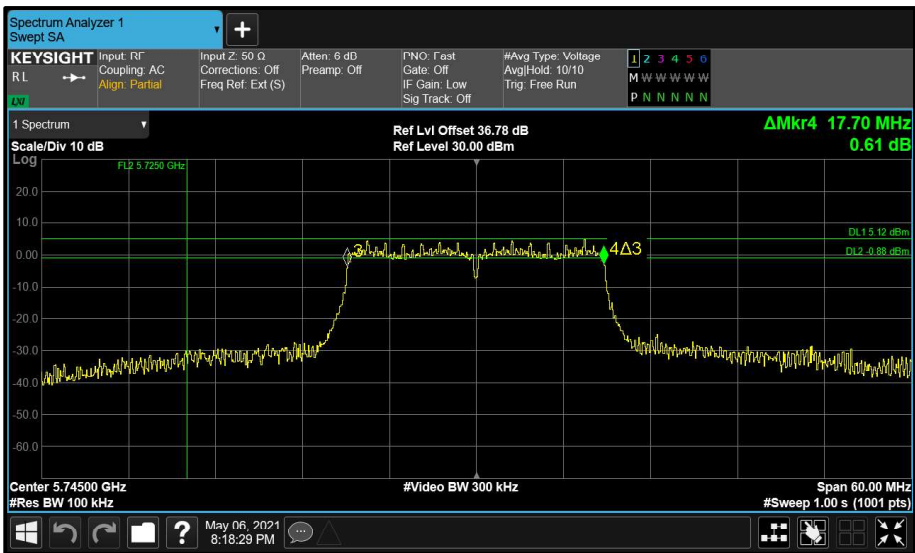
Figure 206 - Main (A) 5745 MHz (CH149) 6 dB Bandwidth
