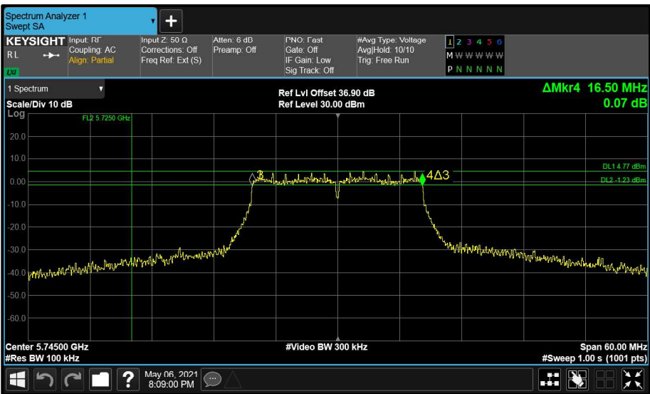
Figure 176 - Aux (B) 5745 MHz (CH149) 6 dB Bandwidth
