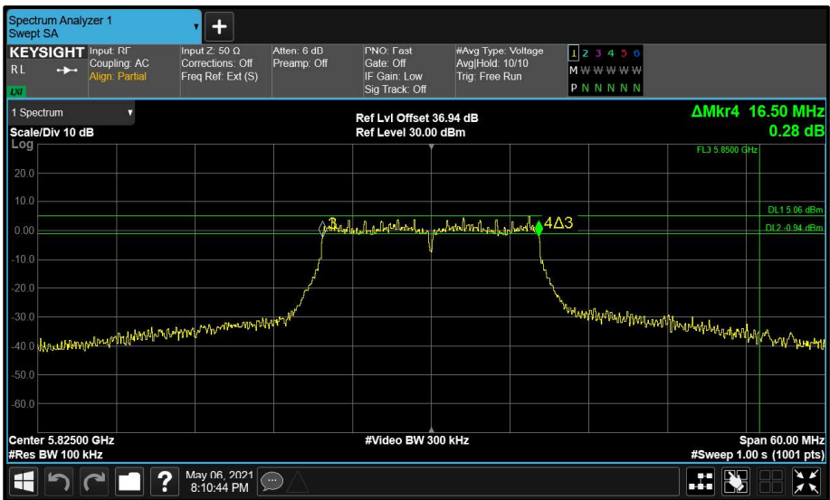
Figure 182 - Main (A) 5825 MHz (CH165) 6 dB Bandwidth
