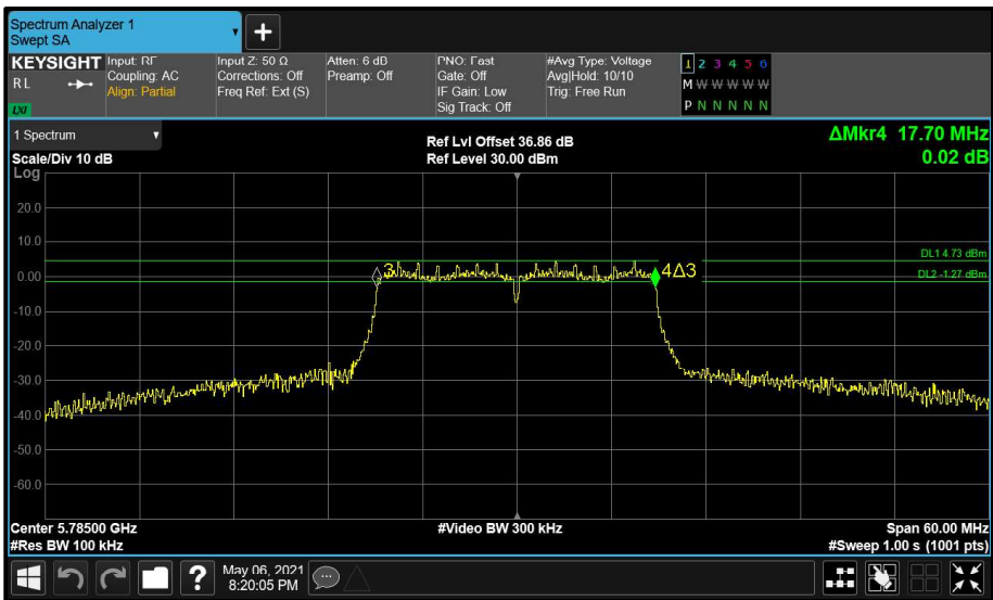
Figure 212 - Aux (B) 5785 MHz (CH157) 6 dB Bandwidth
