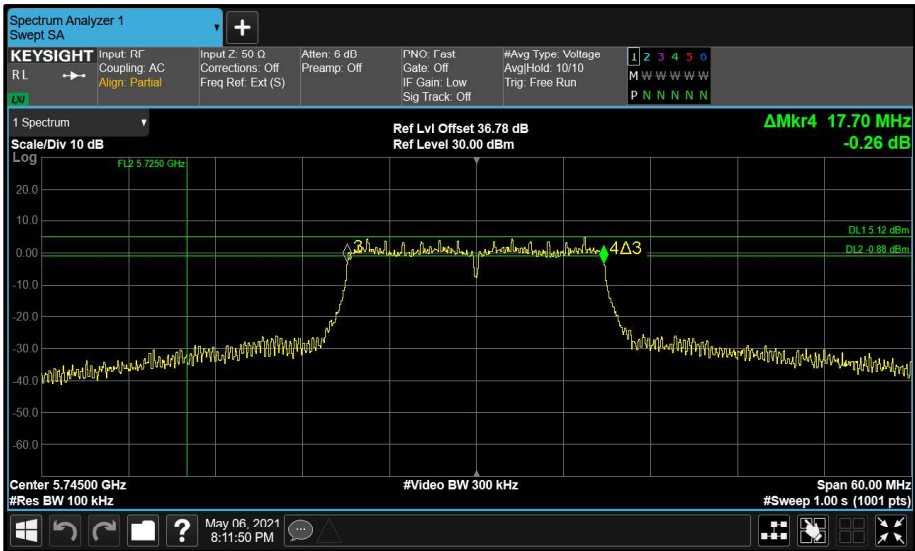
Figure 190 - Main (A) 5745 MHz (CH149) 6 dB Bandwidth
