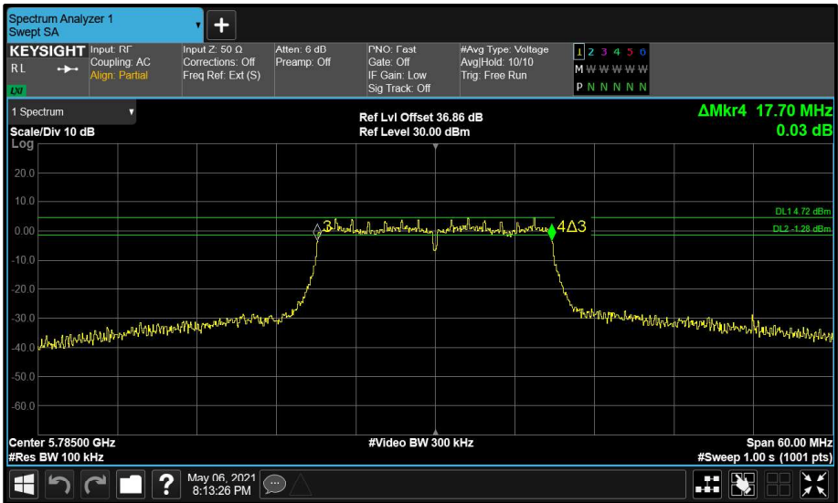
Figure 196 - Aux (B) 5785 MHz (CH157) 6 dB Bandwidth
