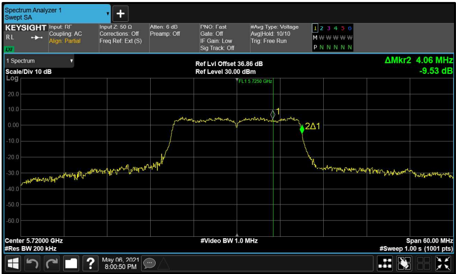
Figure 203 - Aux (B) 5720 MHz (CH144) 99% Bandwidth
