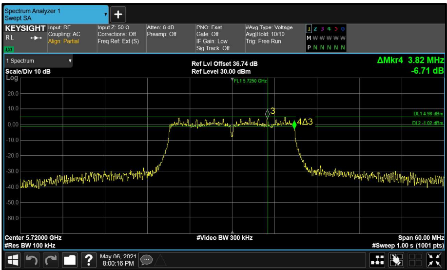
Figure 202 - Main (A) 5720 MHz (CH144) 6 dB Bandwidth
