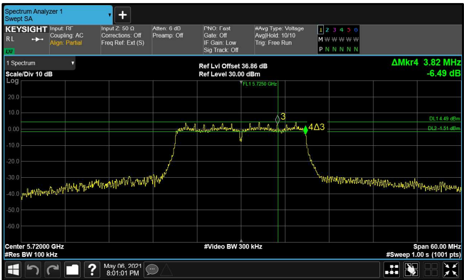
Figure 204 - Aux (B) 5720 MHz (CH144) 6 dB Bandwidth
