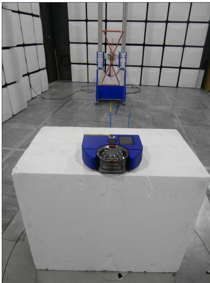
Figure 30 - Test Setup - 30 MHz to 1 GHz
