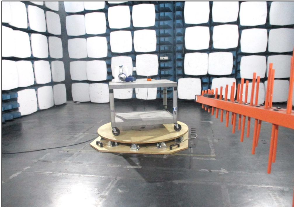
Figure 20 - Test Setup - 30 MHz to 1 GHz - Y Orientation
