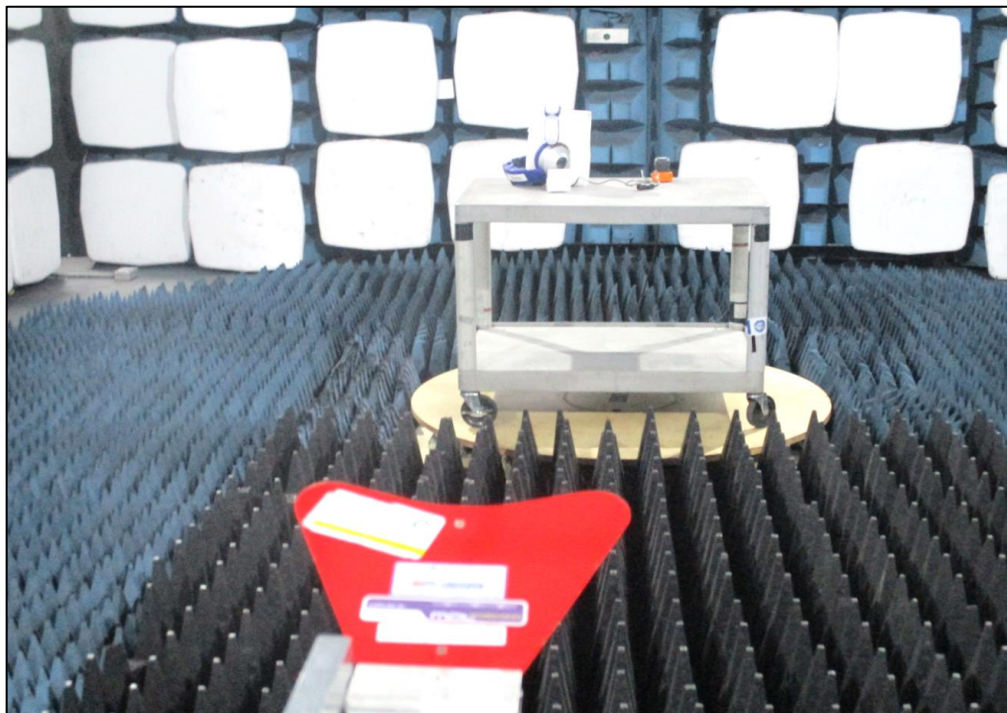
Figure 21 - Test Setup - 1 GHz to 13 GHz - Y Orientation
