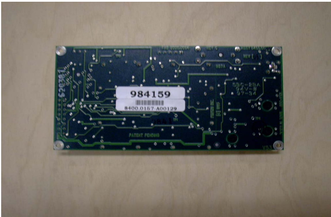
Photograph 5 - 5: Bottom Side of Radio Proxim.
