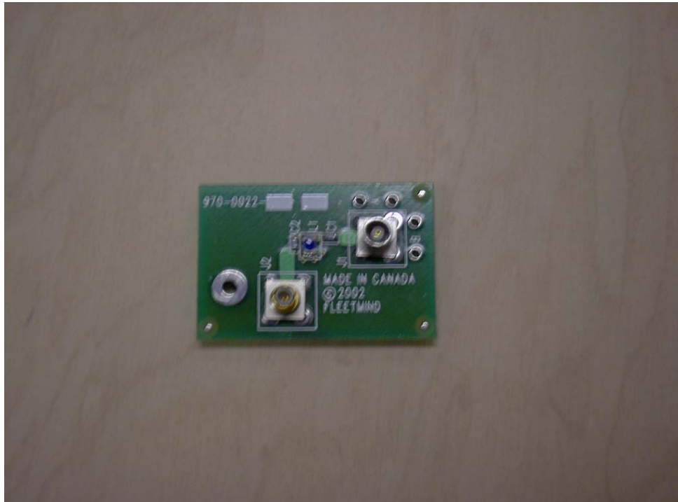
Photograph 5 - 6: Top Side of Filter.
