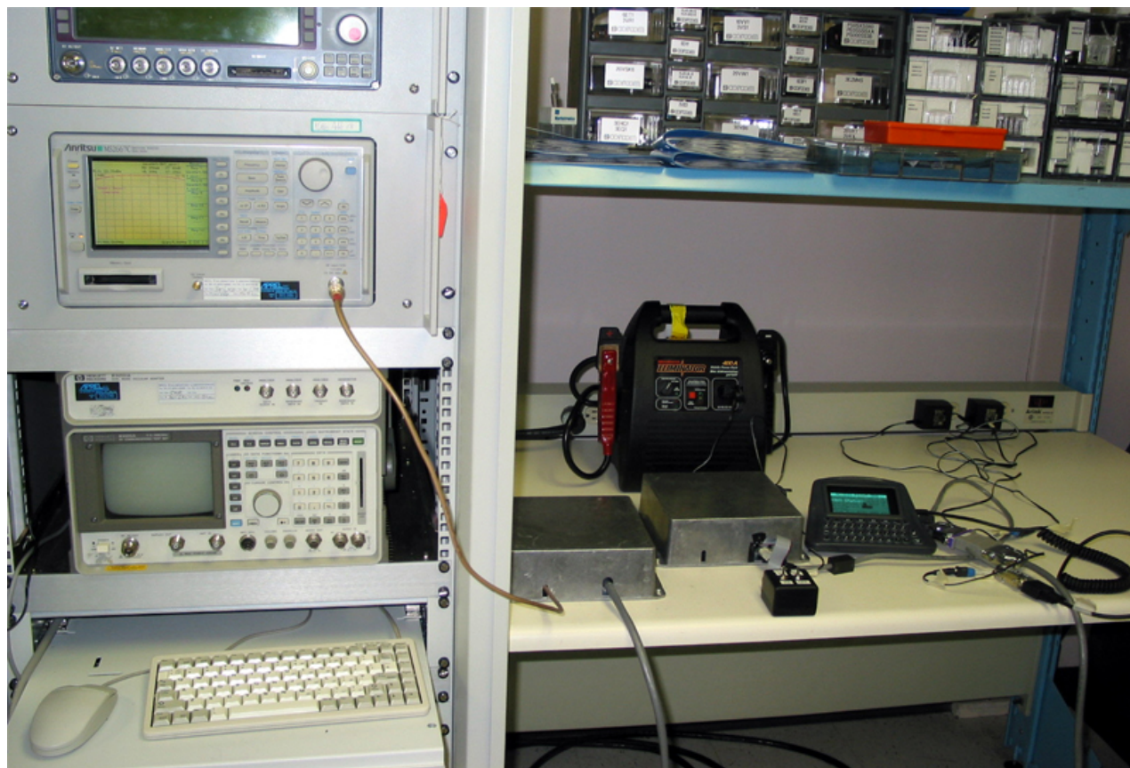
FleetMind – Access Point Maximum Peak Output RF Power Measurement (Conducted)
