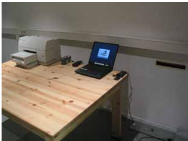
Picture 7 AC powerline conducted emission measurement GSM RX + Computer peripherals
