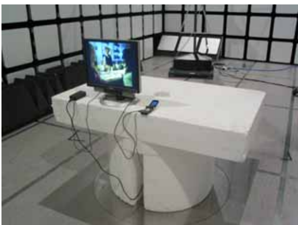
Picture 3 Radiated emission measurement GSM RX +Video
