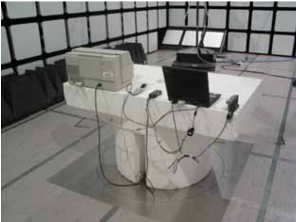
Picture 4 Radiated emission measurement GSM RX + Computer peripherals
