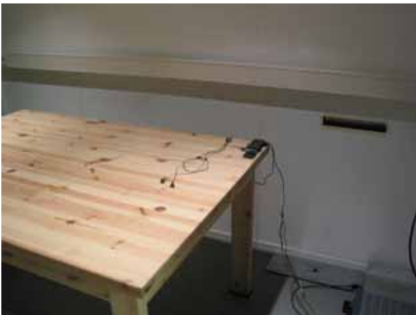
Picture 5 AC powerline conducted emission measurement Bluetooth/WLAN TX + FM radio on
