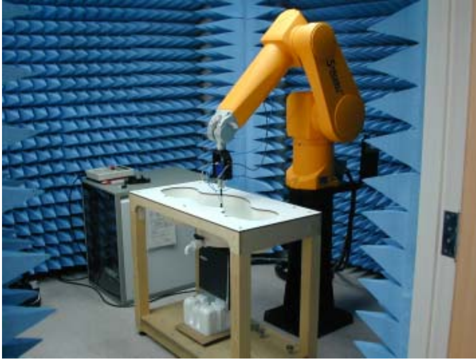
Fig.2 Photograph of the SAR measurement System
