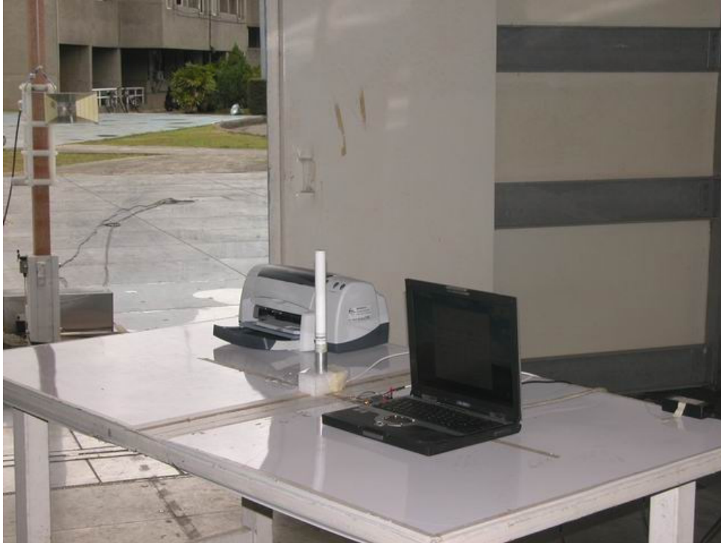
Antenna 3 : Antenna gain is 5dBi
