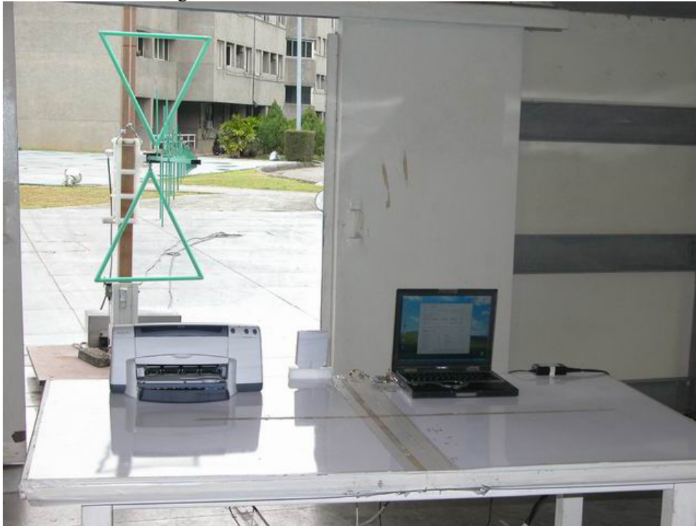
Antenna 6 : Antenna gain is 7.5dBi
