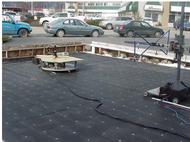
Photograph D.7-2 - 3m ERP Substitution Setup
