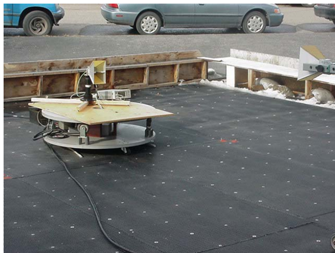
Photograph I.7-2 - 3m EIRP Substitution Setup
