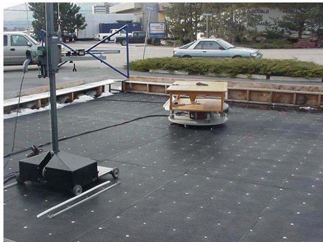
Photograph D.7-1 - 3m ERP Field Strength Setup
