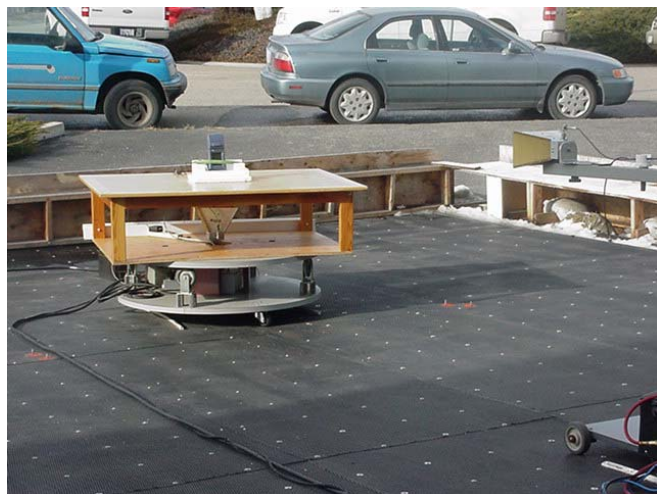
Photograph I.7-1 - 3m EIRP Field Strength Setup
