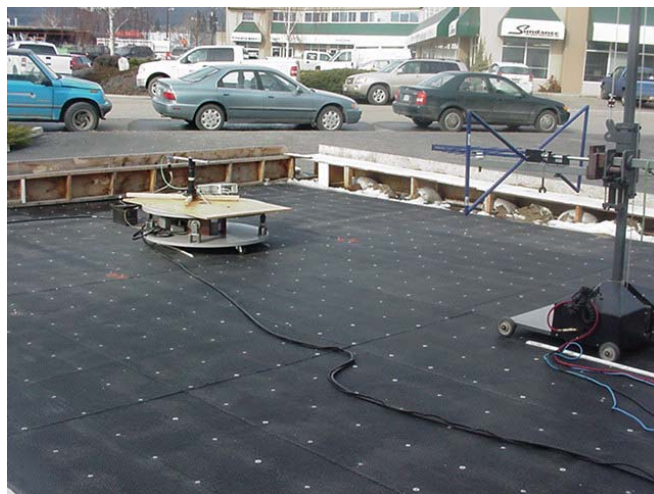
Photograph D.7-2 - 3m ERP Substitution Setup
