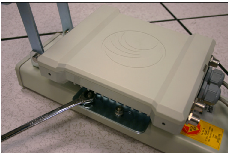
Figure 104 Lower bracket attached to AP antenna
