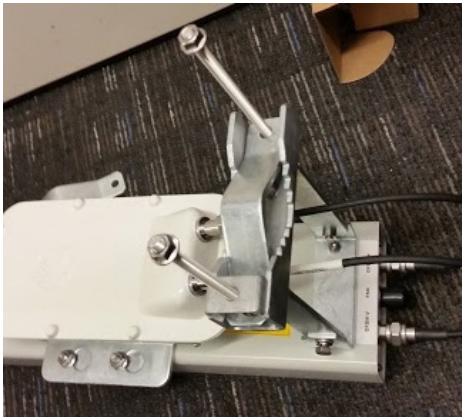
Figure 94 Lower bracket attached to AP antenna
