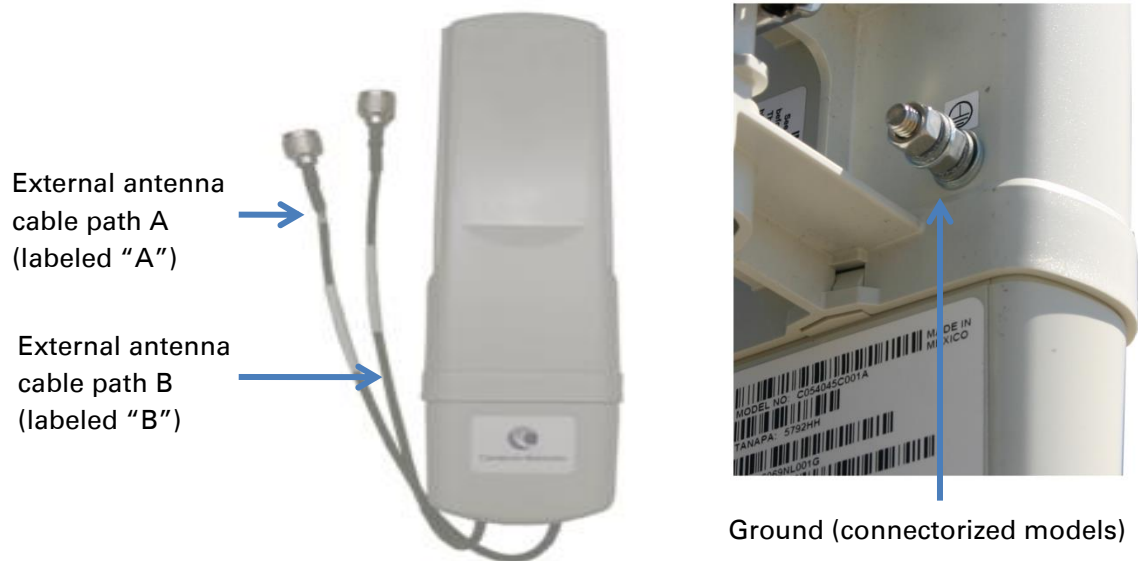
Figure 5 PMP/PTP 450 interfaces – SM/BH Connectorized
