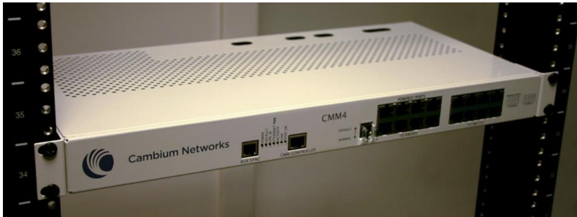
Figure 23 CMM4 (Rack Mount)
