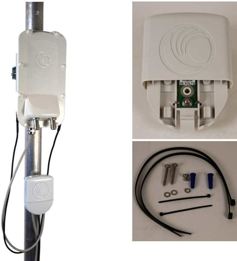
Figure 48 Gigabit Surge Suppressor
