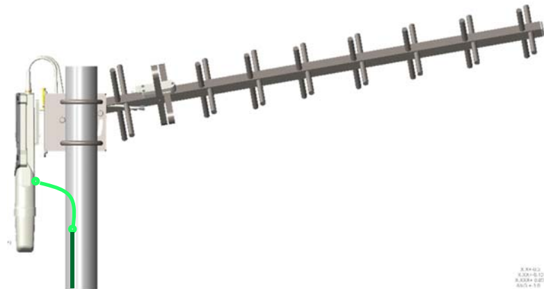
Figure 113 Yagi antenna alignment - downward tilt
