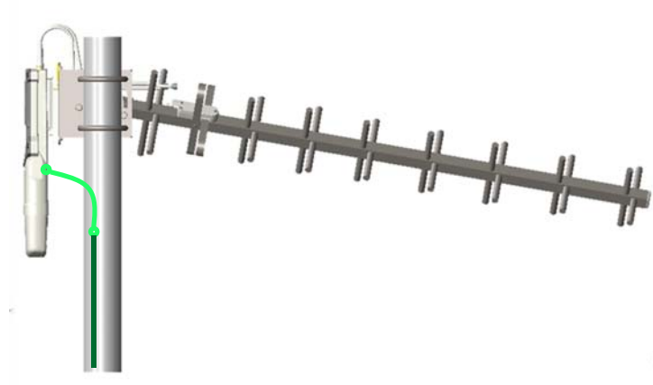
Figure 113 Yagi antenna alignment - downward tilt
