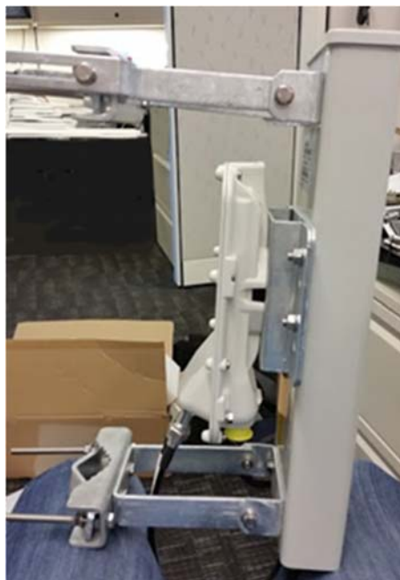
Figure 88 Completed AP and antenna assembly
