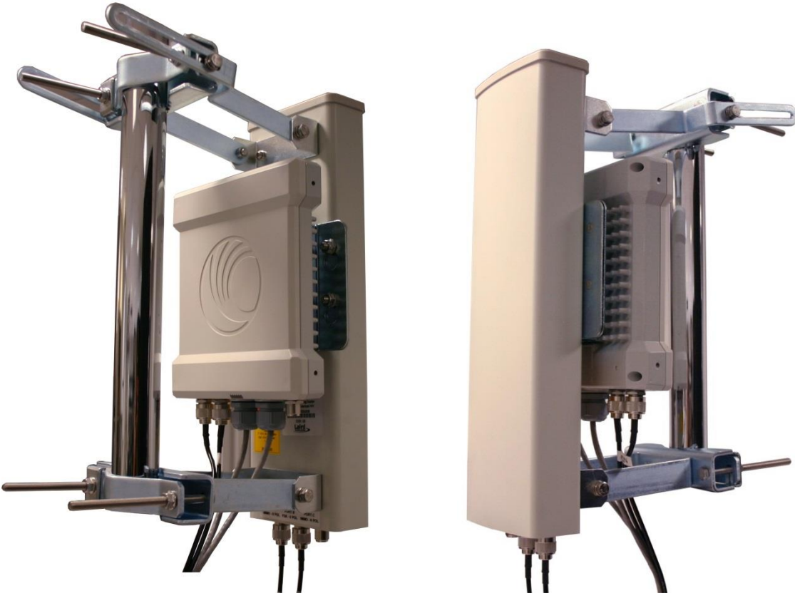
Figure 77 Mounted PMP 450 AP and antenna assembly, viewed from back and back
