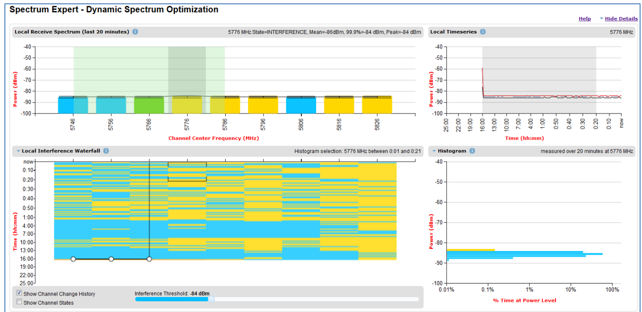
Figure 177 Spectrum Expert page showing the Receive Spectrum, Timeseries, Interference Waterfall and Histogram for the Local unit
