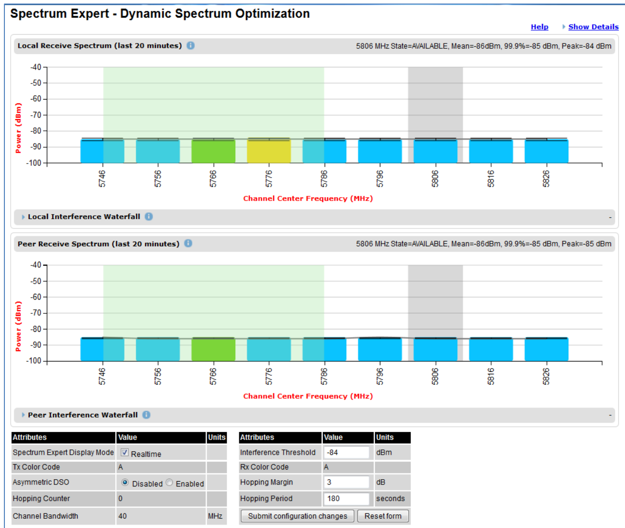
Figure 180 Spectrum Expert page with radar avoidance (Master unit)
