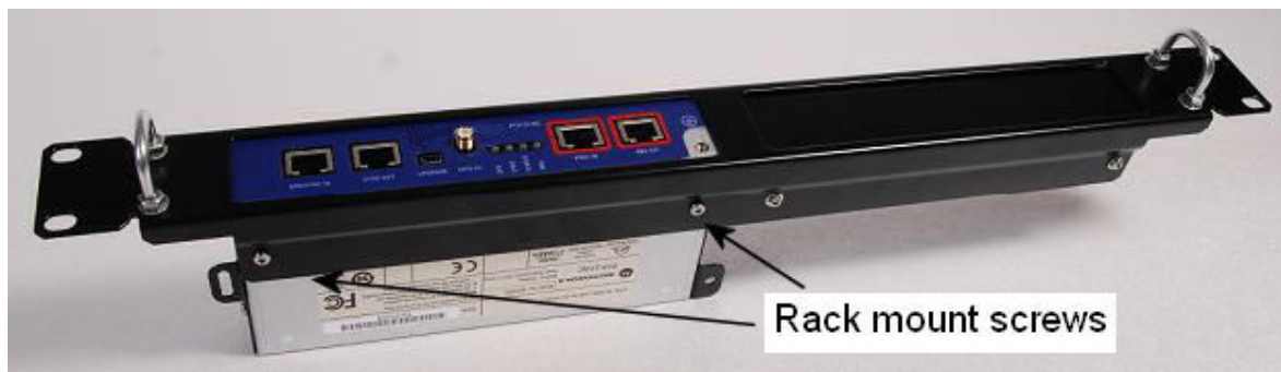
Figure 118 PTP-SYNC mounted in a rack
