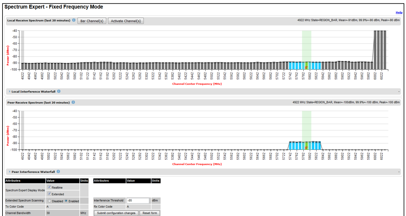
Figure 226 Spectrum Expert page for Fixed Frequency – Extended display mode
