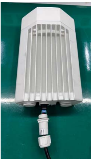
Figure 122: Connecting the input side of AC/DC PSU
