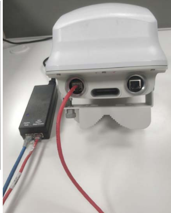
Figure 135: Connecting the V2000 power injector
