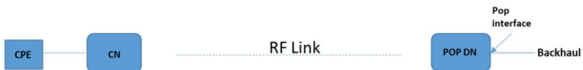
Figure 55: Point to Point cnWave link
