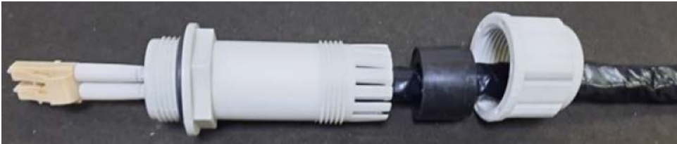
Figure 138: Threading the part onto the cable
