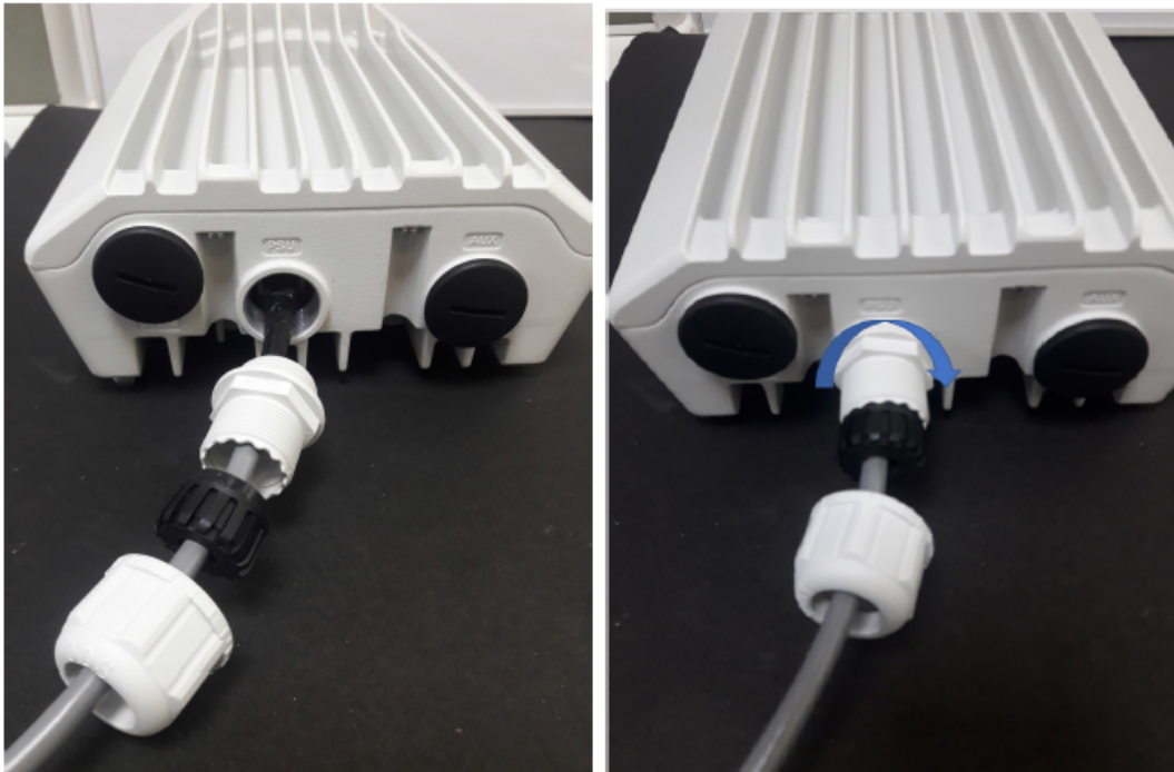
Figure 109: Connecting the RJ45 plug
