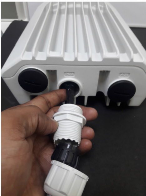
Figure 113: Removing the latch of the RJ45 plug
