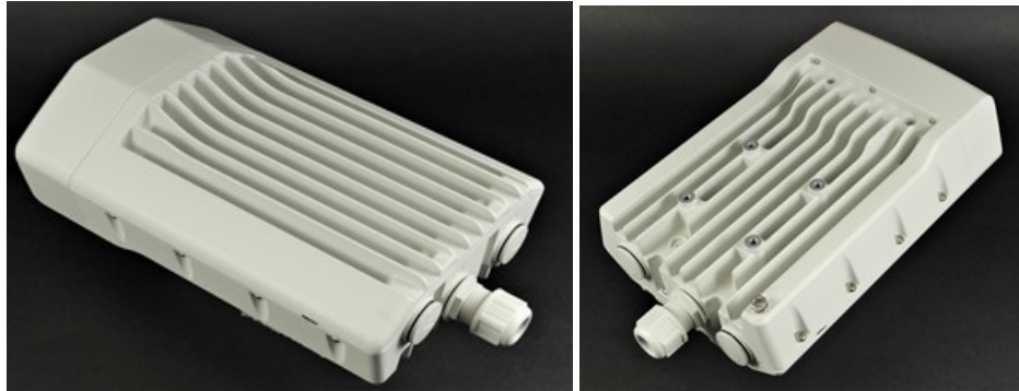
Figure 3 : V5000 Distribution Node front and rear views
