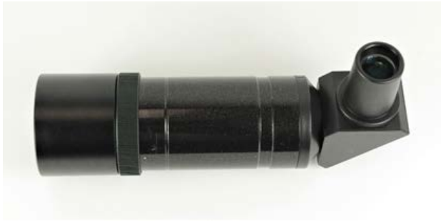
Figure 12 : Typical alignment telescope
