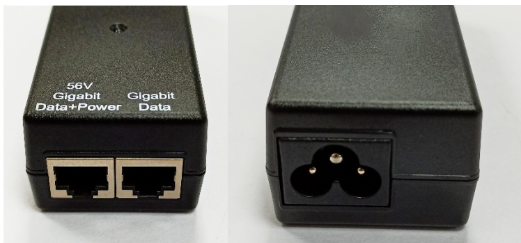
Figure 16: PoE power supply to V1000
