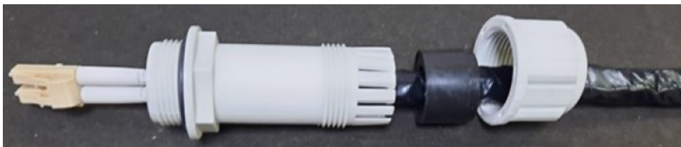
Figure 131: Threading the part onto the cable
