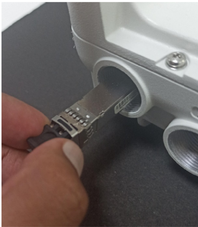
Figure 135: Pushing the module home
