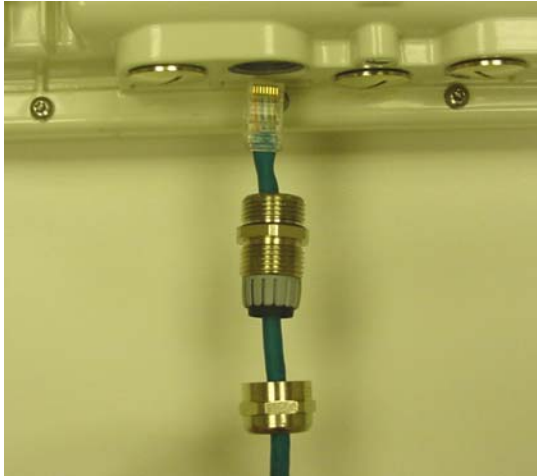
Step 1: Assemble the cable as described in 5.7.1 above
