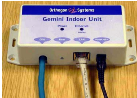
Figure 3 OS-Gemini Indoor Unit (IDU)
