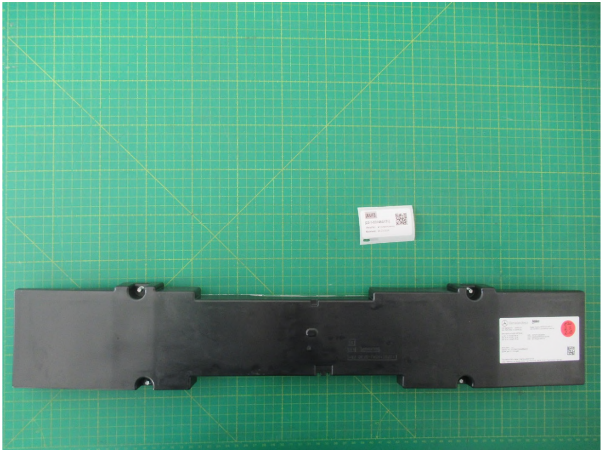
Fig. Ext.: 1 : Ext. - Front Antenna and Remote Telematics Integrated System
