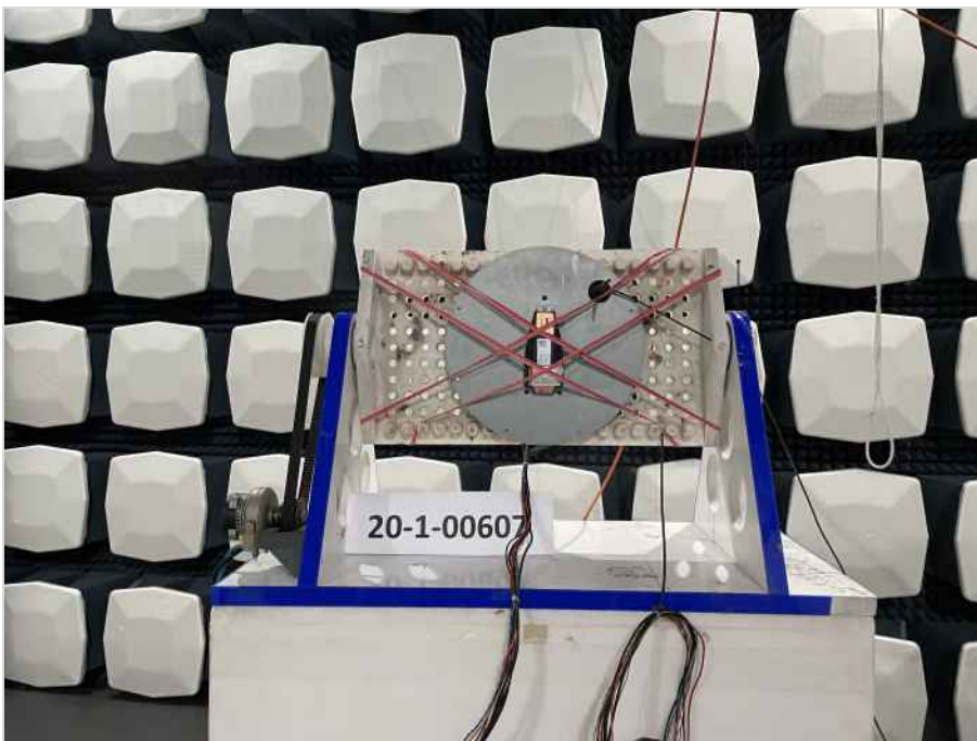
Photograph 2: EUT Test Setup in the anechoic chamber, Radiated emissions
