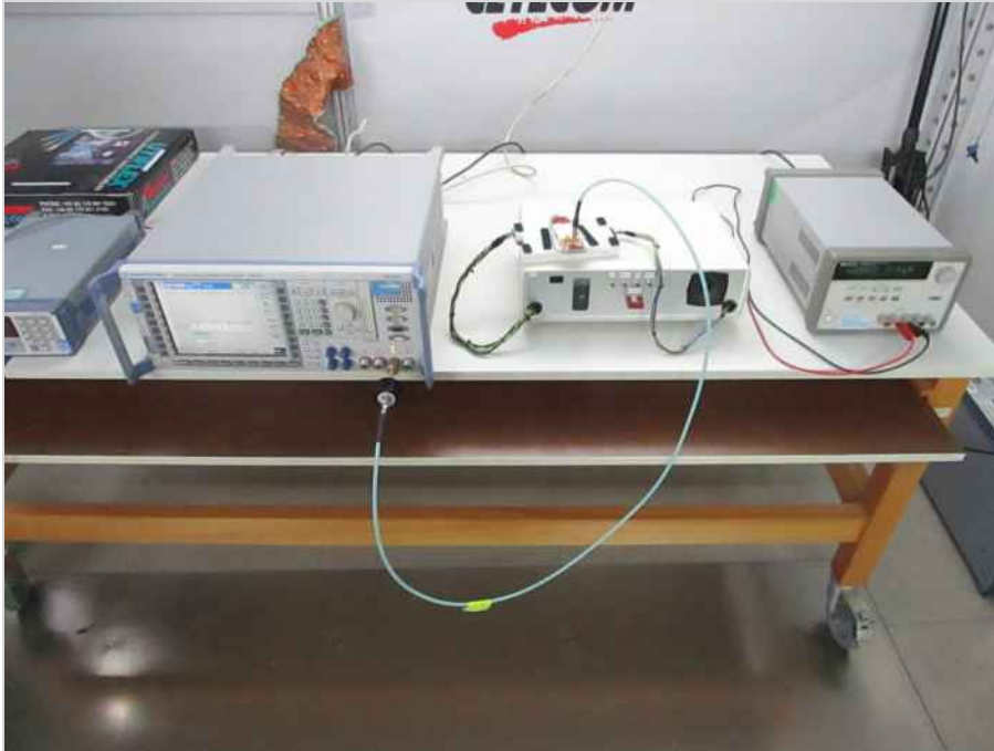
Photograph 5: EUT Setup Conducted RF power
