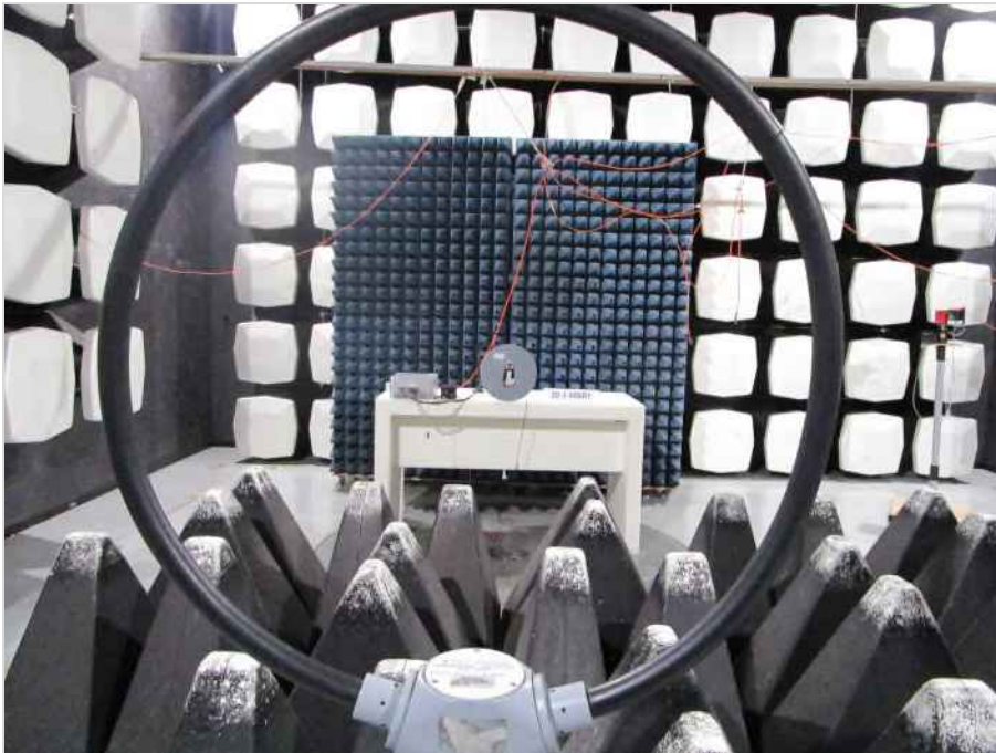
Photograph 3: EUT Setup Magnetic Field Measurements in the Semi anechoic chamber
