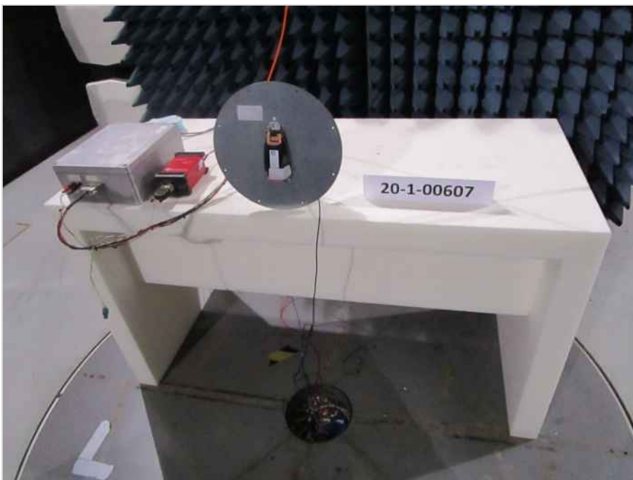
Photograph 4: EUT Setup Magnetic Field Measurements in the Semi anechoic chamber
