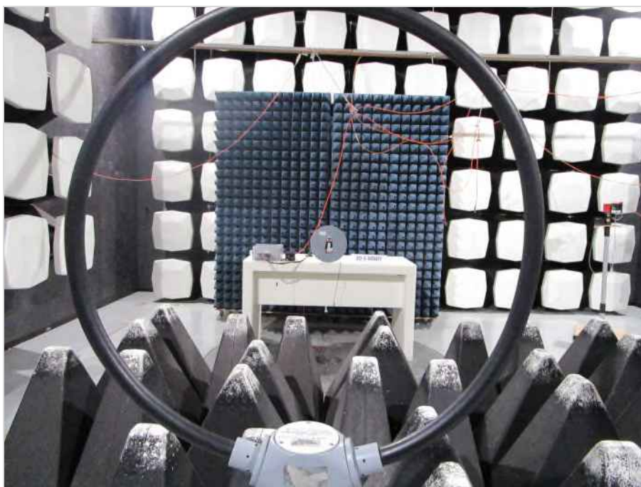
Photograph 4: EUT Test Setup in the semi anechoic chamber, overview
