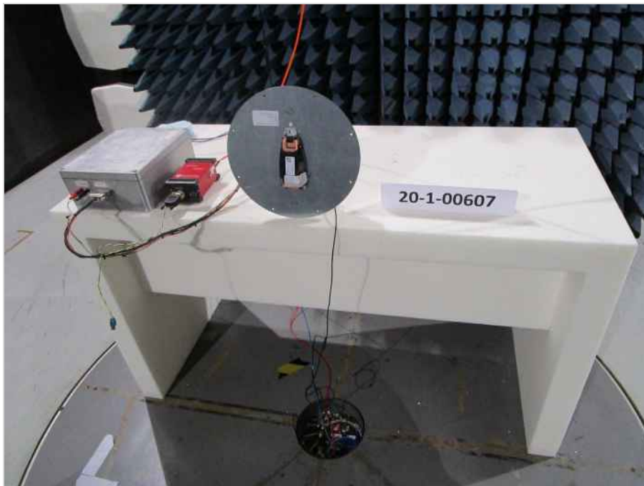
Photograph 3: EUT Test Setup in the semi anechoic chamber, close up view
