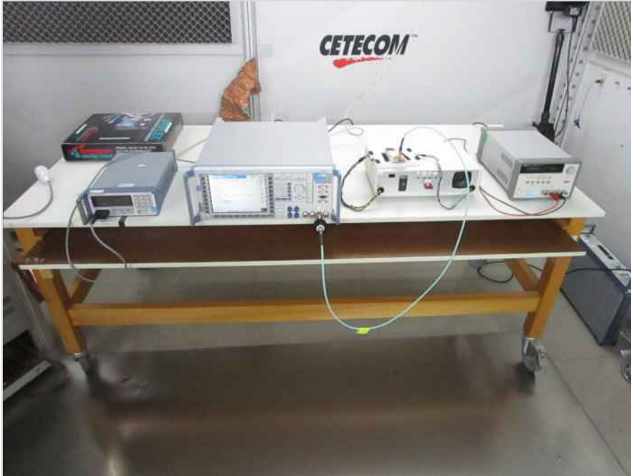
Photograph 5: EUT Setup Conducted RF power
