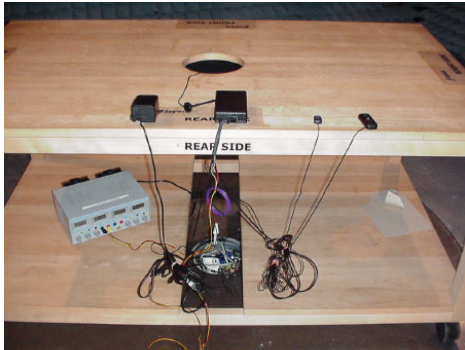
Picture 1 : Setup for the test "Spurious radiated emissions" up to 1 GHz
