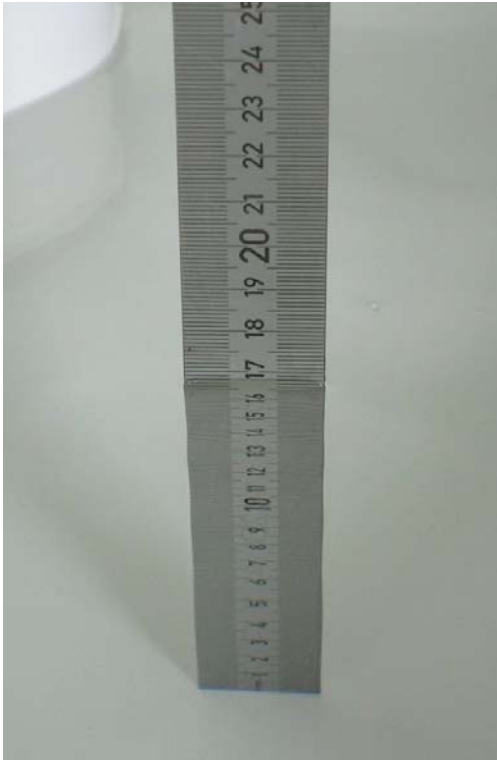
Fig. 16: Liquid depth for Bluetooth body measurements.
