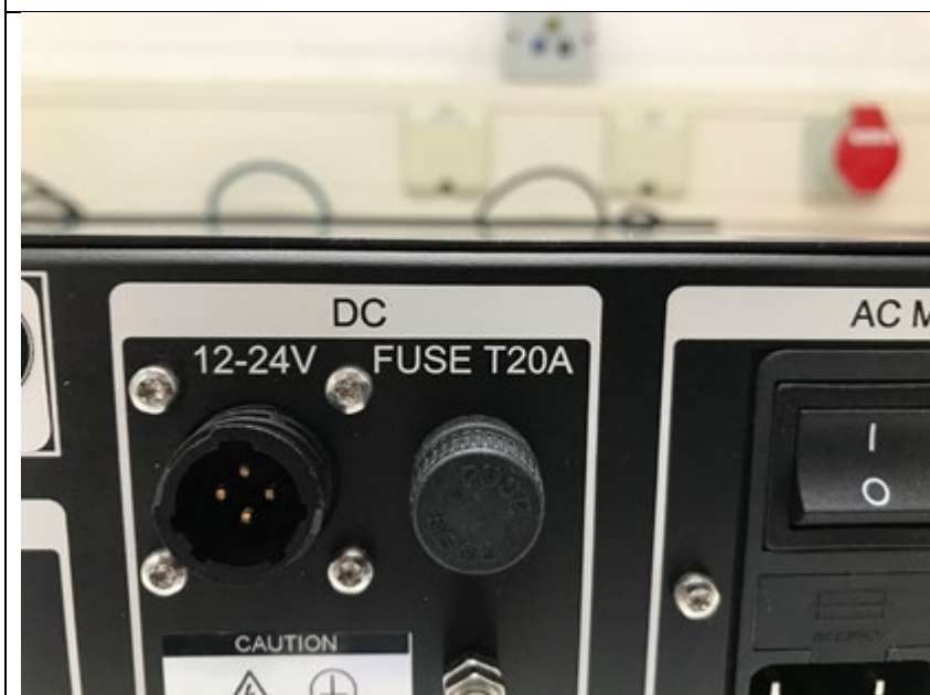
Figure 6: DC Supply connection View
