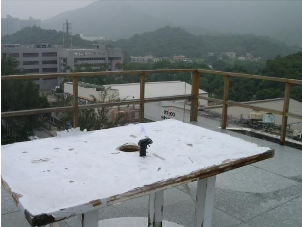
Measurement of Radiated Emission Test Set Up
