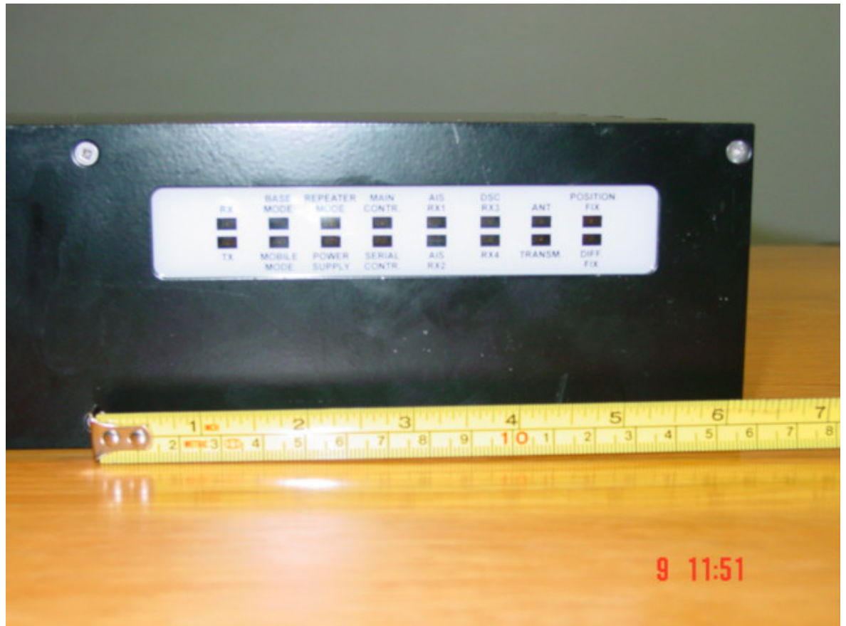
Photograph 5: Front view with leds
