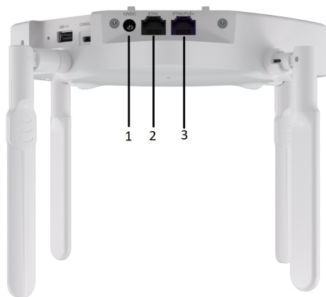
Figure 2: AP3000X Hardware ports
