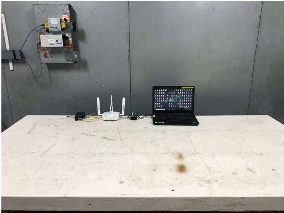
Description: Conducted emission Test Setup(AP305CX)
