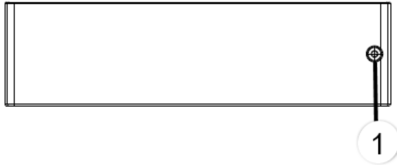
Figure 15: Plastic service panel top captive screw
