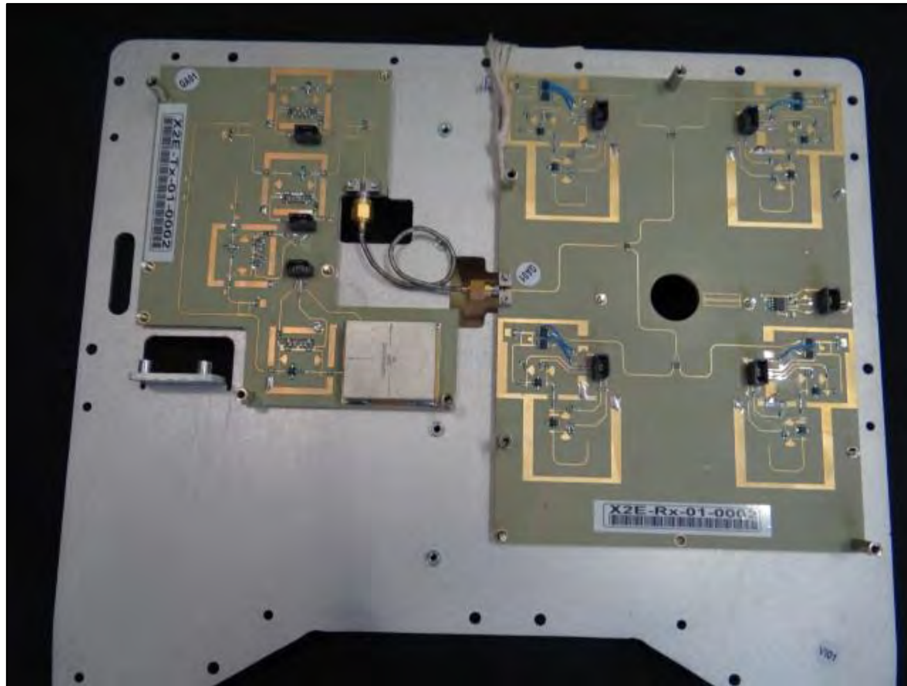
RF Board Component side without shields mounted to carrier plate.
