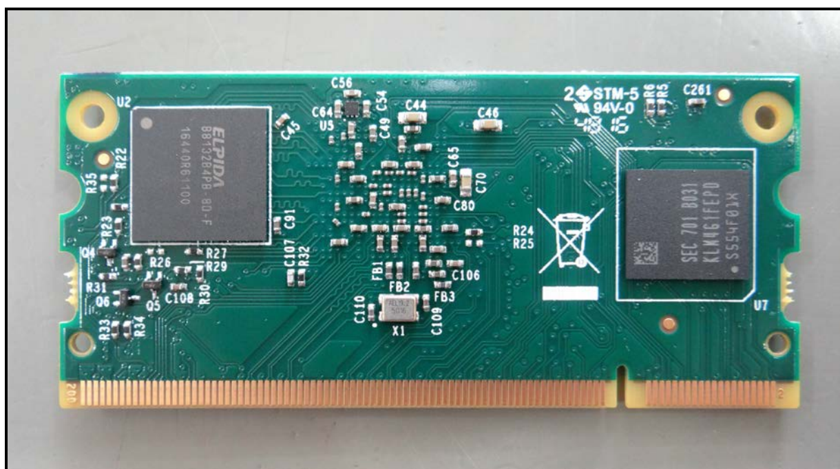
Raspberry Pi Compute Module 3 Bottom Side
