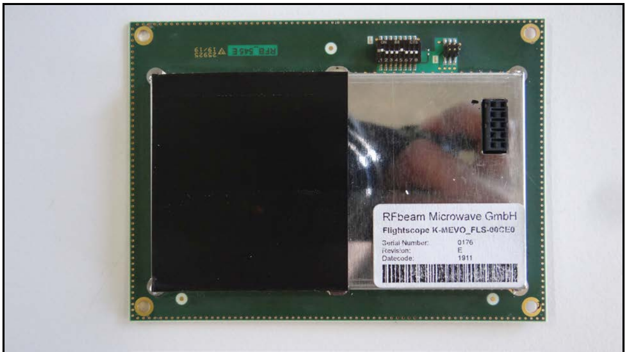
Microwave Board Assembly Bottom Side
