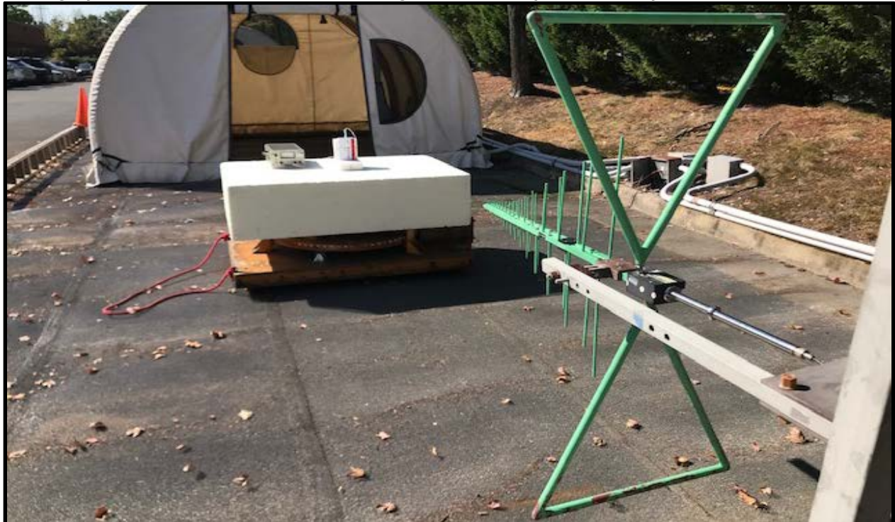
Photograph 1: Radiated Emissions Testing – Front View (Below 1 GHz)
