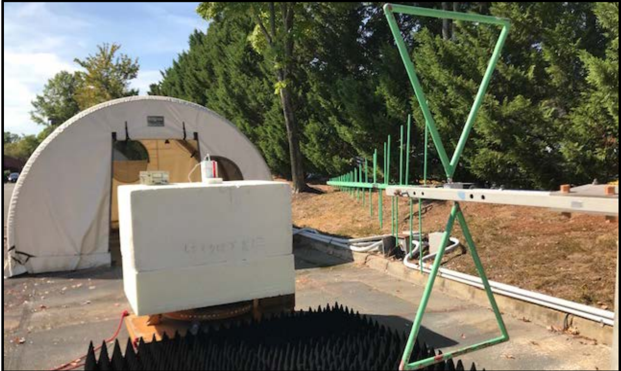
Photograph 4: Radiated Emissions Testing – Rear View (Above 1 GHz)
