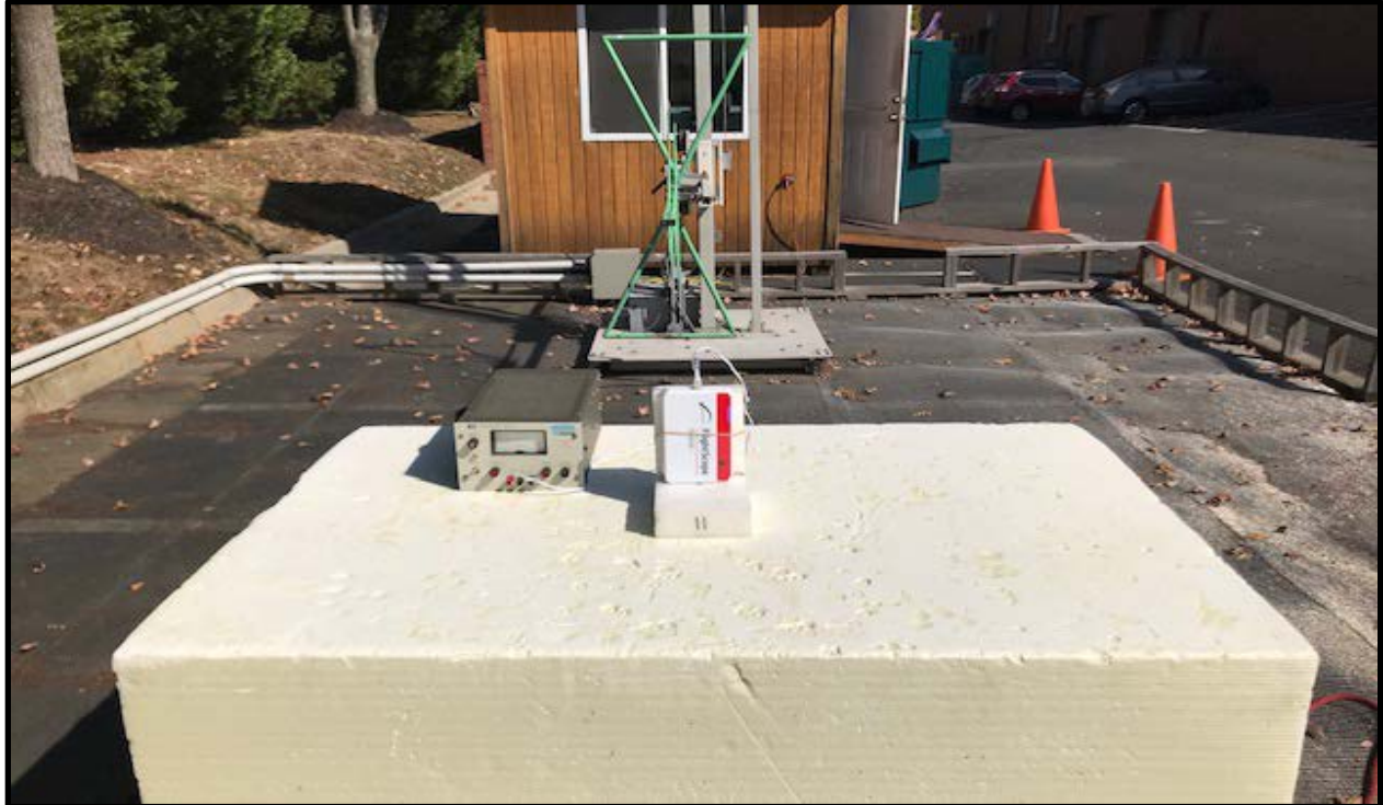
Photograph 2: Radiated Emissions Testing – Rear View (Below 1 GHz)
