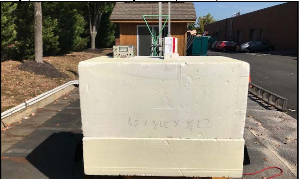
Photograph 4: Radiated Emissions Testing – Rear View (Above 1 GHz)
