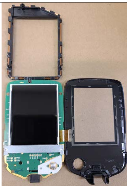
Photo 2- Internal Top View of Reader with Bobbin Removed
